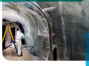
Aquaria, monolithic blocks in methacrylate (PMMA) chemically treated and produced for specific use in the underwater field.
